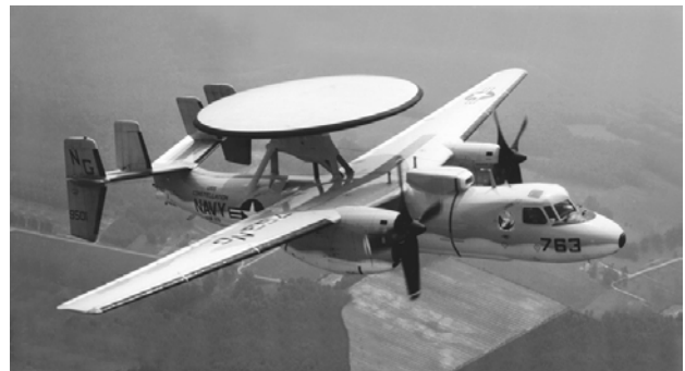
Figure 2. For effective communications, some aircraft such as the E-2C Hawkeye may require sophisticated adaptive processing systems such as co-site interference management systems. Use of software-defined radio communication systems in such aircraft requires use of software-defined antenna and interference management systems. (Figure: Northrop Grumman)
