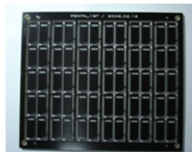
Fig.3. Antennas manufactured by PCB technology.
