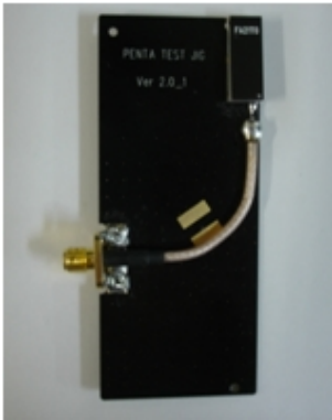
Fig.4. The installation of antenna to test jig.
