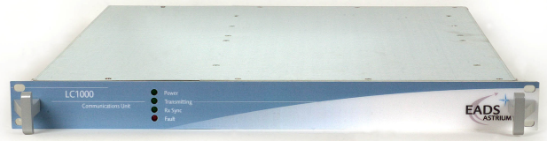
Figure 4: The LC1000 Modem – Astrium's Low Cost COTS SDR Platform
