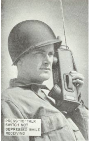
Radio Set SCR-536, the smallest Signal Corps transmitter/receiver of World War II.
